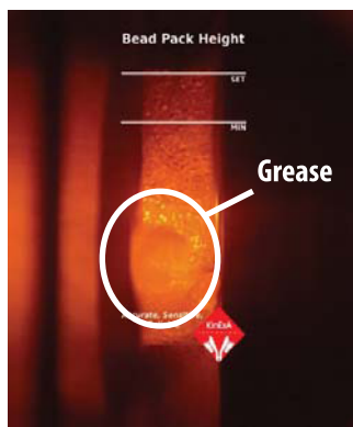
Figure 1. Flow cell image obscured with excess grease
