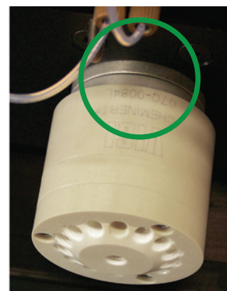
Figure 2b. Valve is fully seated.
