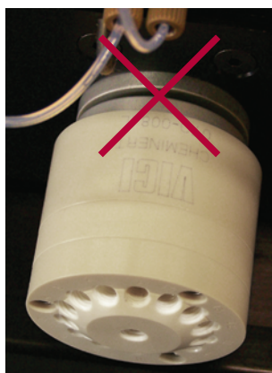
Figure 2a. Valve is not fully seated.
