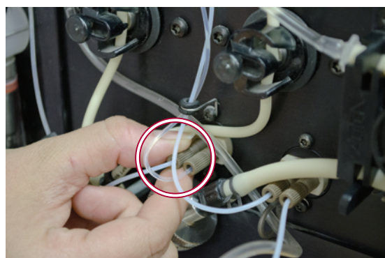
Figure 2. Disconnect the nut from the left side of the solenoid valve on the left.
