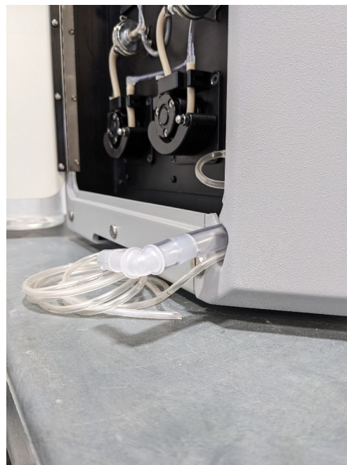
Figure 6. Buffer Line and Waste Line Elbow.
